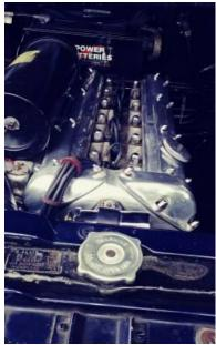
many Jaguar Drivers and Restorers Club events. 3.4L inline six cylinder double overhead cam engine, dual SU carbs. New porcelain exhaust manifolds. Rebuilt and re-sleeved brake master cylin-
